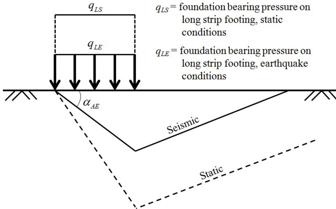
Figure 4. Shear failure surfaces of foundations for static and seismic conditions (Richards et al., 1993).
