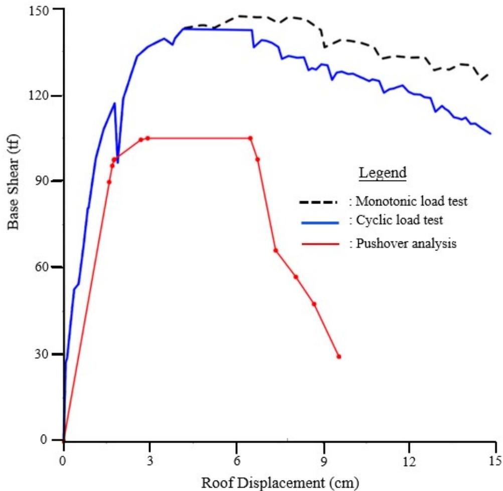
Figure 9. Capacity curves obtained through pushover test analysis (Chung, et al., 2013).
