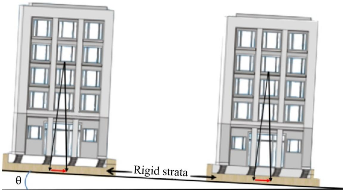
Figure 16. Vibration-isolated buildings tend to be unstable on a rigid stratum inclined during a severe tectonic earthquake.
