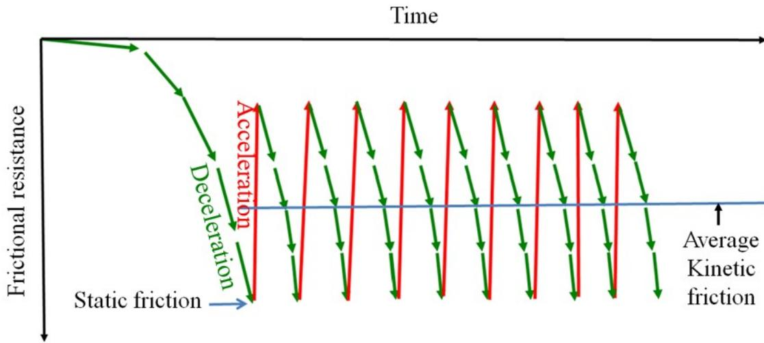
(c) Repeated stick-slip phenomenon induced by shear banding (Lambe, 1969).
