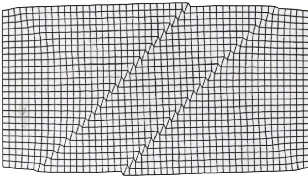
(b) Shear bands induced by localizations of deformations (Hsu, 2018)
