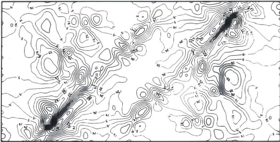
Figure 11. Highly concentrated excess pore water pressure induced by shear zone dislocation (Hsu, 2018).
